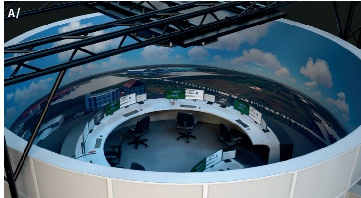
A/ Front projected solution 6 projectors 38° Vertical Field of View
