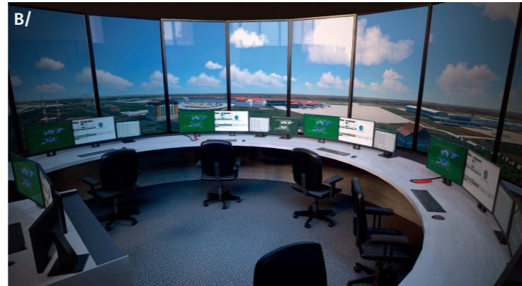
B/ Monitor projected solution 24 monitors 24° Vertical Field of View
